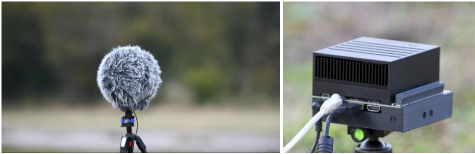
Figure 4: View of an acoustic sensor with its protective windshield and a local processing unit
