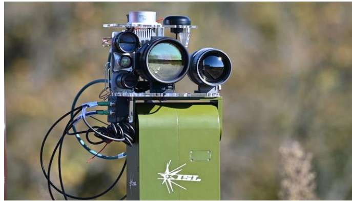
Figure 10: Acoustic array, E/O system deployed during the experiments
